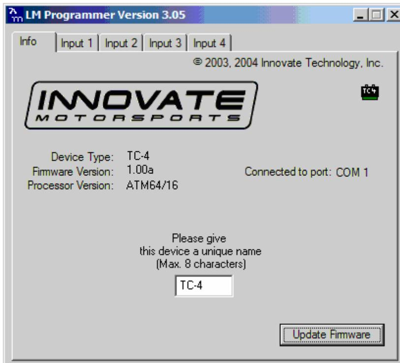
The LM Programmer software then shows in its first page the type and version number of the firmware of the device.
