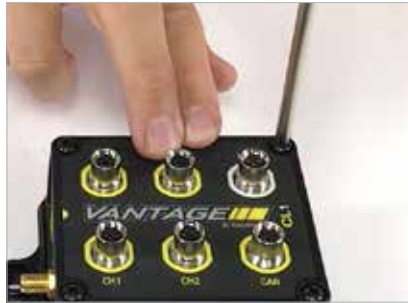
8. Reinstall the four screws, taking care to not overtighten.
