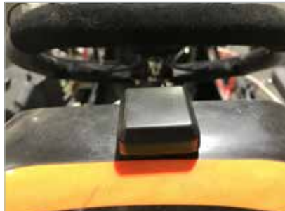
5. Racepak suggests mounting the GPS antenna on the top of the front panel.
