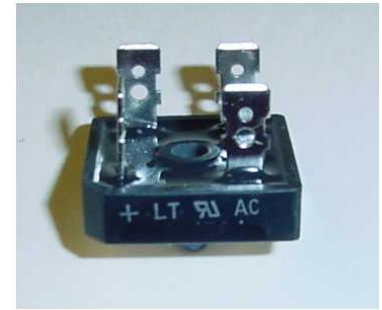
rectifier markings on the side
