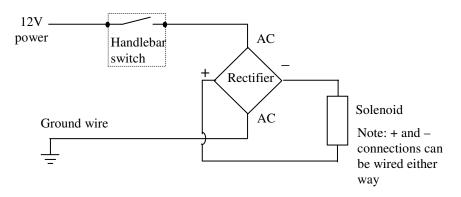
2. Mount the rectifier to the air box. Use the picture to identify the beveled corner on the rectifier so the terminals (+, AC, -, AC) can be identified.
