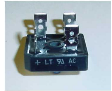
Rectifier markings on the side
