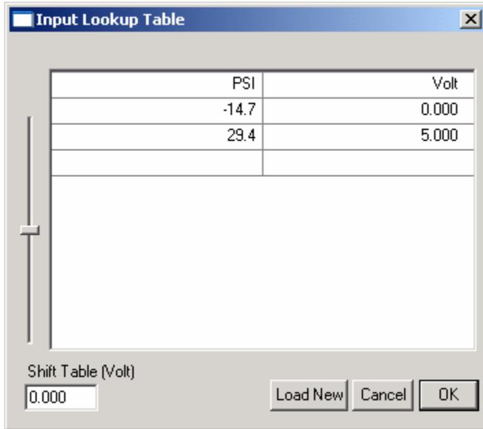
Double click on any field in the table to modify it. Click on a field to select it. To delete an entry, select it and hit the delete key.
