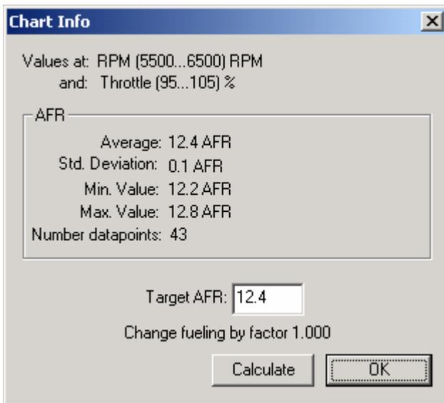
This shows the current values of the clicked field. The target AFR or Lambda calculation functions are only available if the field content is AFR or Lambda. The fueling change calculation is based on fuel flow control where higher numbers represent more fuel. If for example your EFI is set by injector timing, just multiply the timing setting by the suggested number.
