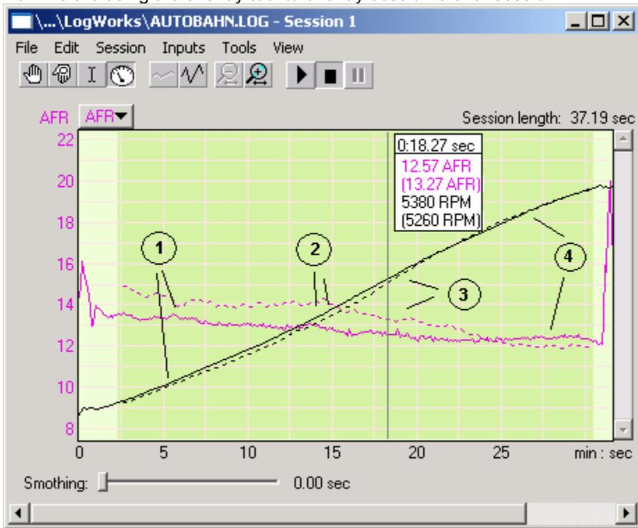
What is immediately noticeable is that the AFRs of session 3 are higher than those of session 1 in the area below 7000 RPM, but lower above. Let's see how that affects power and acceleration. Acceleration can be determined by the slope of the RPM curve. The steeper the slope, the higher the acceleration and therefore power (assuming other conditions like weight and wind are the same).
