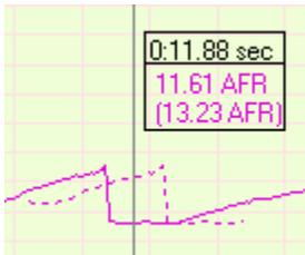
Using the overlay scroll tool you can move the overlay left and right. If a measurement point overlaps an overlay trace, the overlay measurements at this point are shown in brackets (). The hand tool or horizontal scroll bar moves underlying graph and overlay together. Overlays are not saved with a log.
