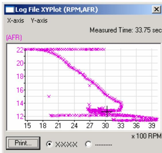
In this case the Y-axis is AFR and the X-axis is RPM. You can select any two inputs as either of the X or Y axis. If nothing in the graph is selected, the X-Y Plot represents the data of the entire session. If a part of the session is selected (Selection Tool), only the data of the selected areas is represented.
