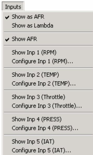
This menu allows switching mixture display between AFR and Lambda. It also allows selectively switching input traces on and off and configuring the inputs.
