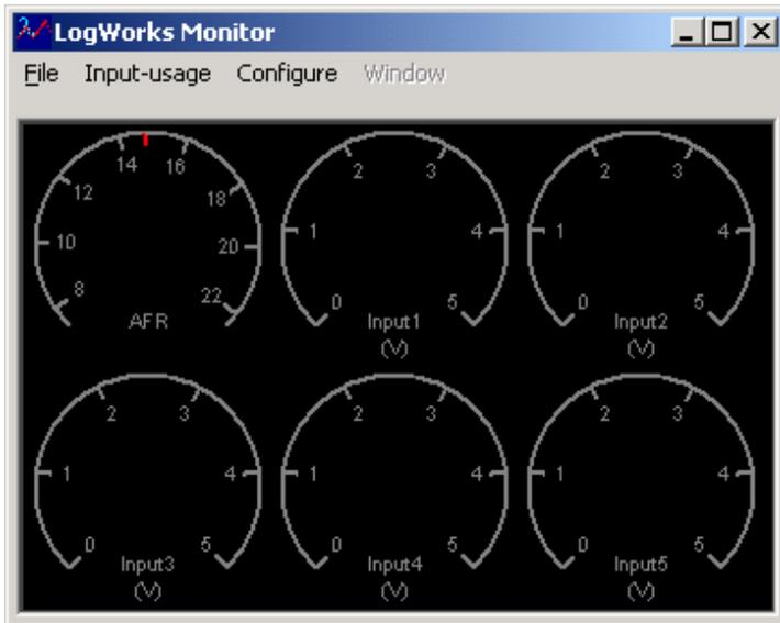
This window is resizable by grabbing on the lower edge of the window. The round gauges are typically arranged in a 3 x 2 arrangement. This arrangement will be changed depending on the window width and height to maximize the gauge size. All gauges are greyed out until:
