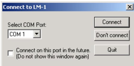
Select the serial port (COM Port) to which the LM-1 is connected. Then press the Connect button.
