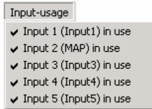
Allows selectively switching inputs off that are not connected or not used for datalogging. The appropriate gauge is grayed out when switching the input off and the data from that input is not used or shown in the real-time log or LM-1 log.
