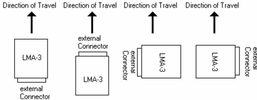
The mounting position should not deviate more than 3 degrees from horizontal.
