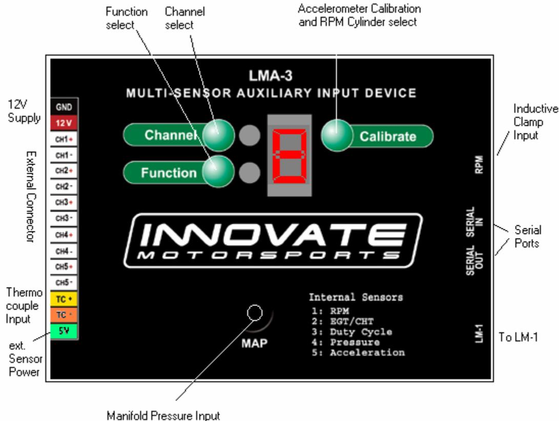
Plug the supplied Mini-DIN8 to Mini-DIN8 cable in the LM-1 port of the LMA-3. Plug the other end of the cable into the AUX-IN port of the LM-1.
