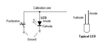
Any color LED can be used. A typical LED has 2 wires called Anode and Kathode. The Kathode side is the shorter of the 2 wires. It is connected to Ground. The Anode side will be connected to the calibration wire.
