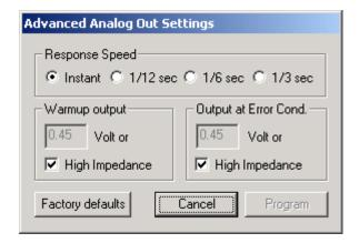
When setting the LC-1 to the slower response speed settings the measured mixture data will be averaged over the response time setting before being output.
