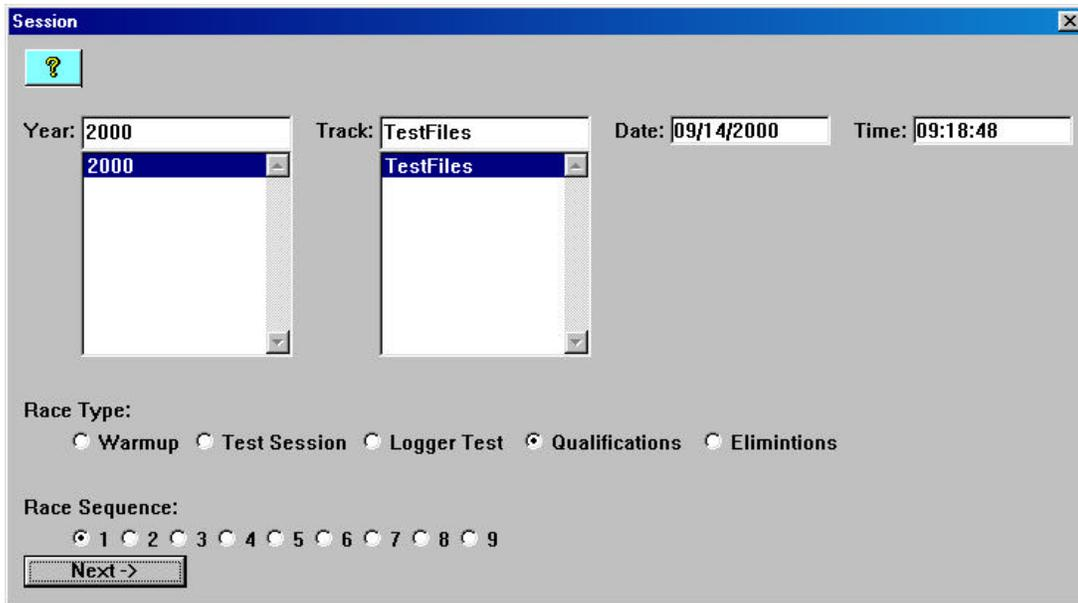
Select **OK** or **Next** depending on your configuration file. Additional dialog boxes may be displayed. These are part of the Run Log sections that are user programmable to allow test information to be entered during the download process. Fill out the information as appropriate. The file save dialog box will then be displayed as shown below.
