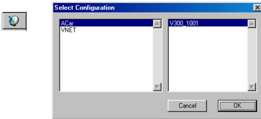
Select the configuration file as setup above. A dialog box will then be displayed to allow you to enter the session information (the same as when uploading run data). Enter the appropriate year, track, race type, and race sequence information as shown below. The system will enter the date and time.
