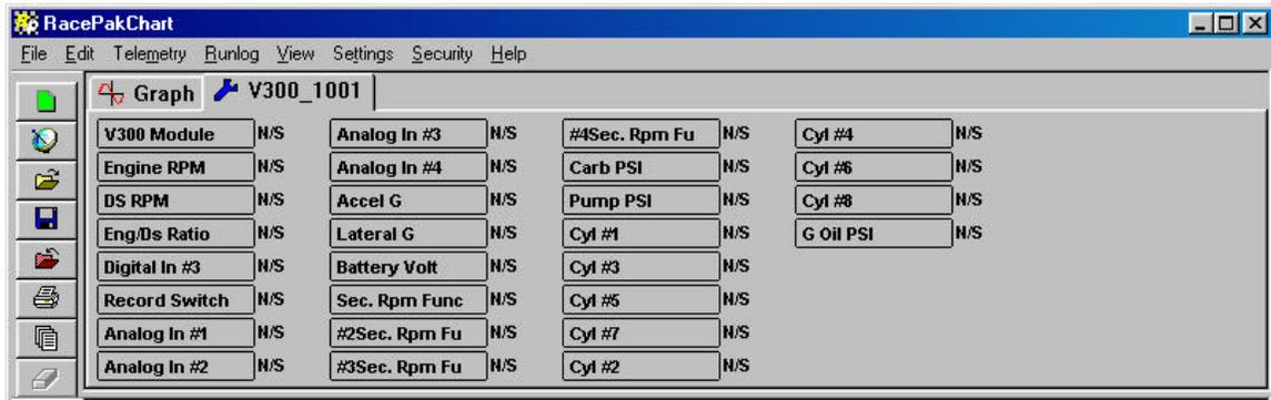
The wrench icon in the run file tab is used to indicate that this file is a car configuration file. Each of the buttons represents one of the devices/channels in your system. For instance the V300 Module button represents your data logger, the Engine Rpm button represents the engine rpm channel, and the G Oil PSI button represents an oil pressure gauge in your system.
