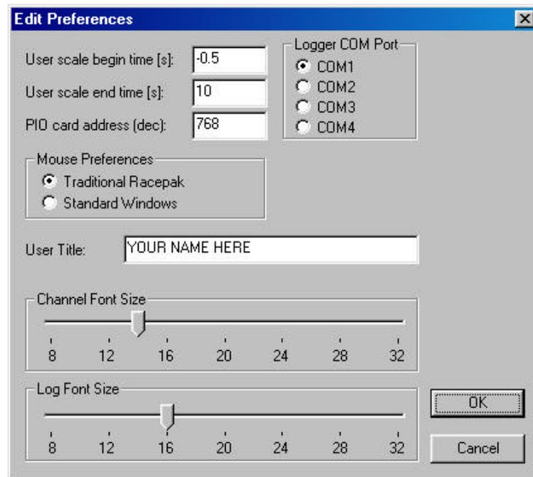
Locate the **Logger Com Port** selection box and select the communications port to which the serial communications cable is connected. Next select **OK** to accept your selection.
