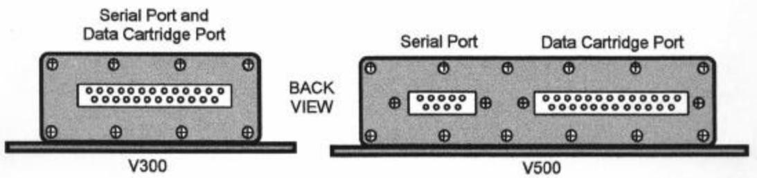
The serial communications connector (or serial port) is used to connect the data logger to your PC computer. When connected, your PC can be utilized to setup or program the data logger, download the information recorded by your data logger, or be used to view and record real time data from the data logger. Each of these functions will be discussed in detail later.
