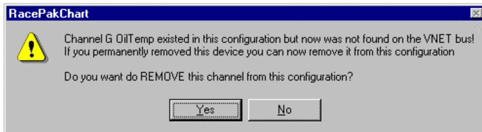
If you have removed the module from the system you should select **Yes** to remove the module from the configuration file. If you have not removed the module from the system you should select **No** and then inspect your system to be sure the module is properly installed. When you have corrected the problem you should repeat the process above.
