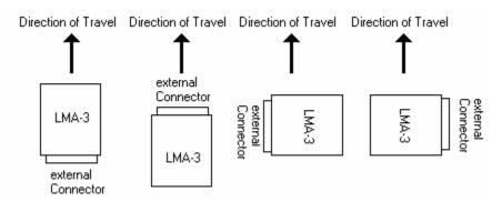
The mounting position should not deviate more than 3 degrees from horizontal.
