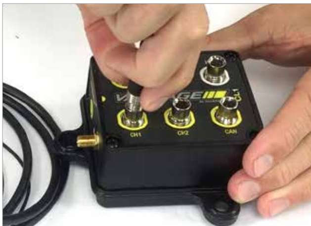
3. Snugly finger tighten the cable connector to the CL1.
