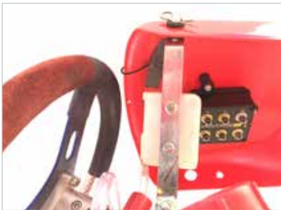
4. Racepak suggests mounting the CL1 under the top of the front panel.
