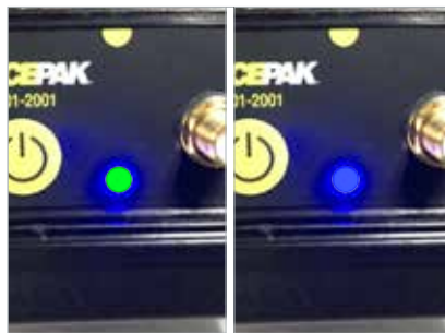
11. The status LED on the CL1 will now alternate between green and blue, indicating the CL1 data box and mobile device are paired and ready for use.
